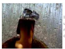
In shoulder stopped locks (almost all modern locks qualify), continued use will cause light impact marks along the face of the plug. This is normal, and should not be confused with the extreme material displacement that occurs during <u>key bumping</u>.
