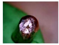
The pins inside this lock show heavy damage from where the screwdriver or chisel was forced into the keyway. Examination of what is left of the tip of the pin shows no indication of covert entry techniques. Because of the force used, tool marks on the pins are rather distinct and may later be used to link suspects to the crime.
