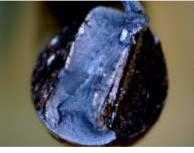
A closer examination of the tool mark reveals that a red substance is present in the area where the bolt cutter was used. This could be a variety of things; paint, dirt, grease, or rust. We might be able to match this material to the tool if a bolt cutter is found in a suspect's possessions.
