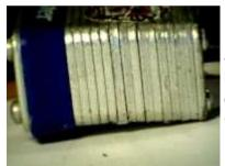
A thorough examination of both the shackle and the padlock body helps to identify the specific technique used. In this photo, the body of the padlock shows excessive distortion in the form of twisting, indicative of extreme torsion being applied to the padlock body.
