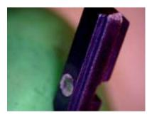
Many unskilled attackers may attempt to bump unbumpable locks. This will probably damage the lock and borders on breaking the lock completely. In the photo, an EVVA 3KS wafer is shown after an bumping attempt. The wafer arm has broken off and a large dent is present, this lock was non-functional after this.
