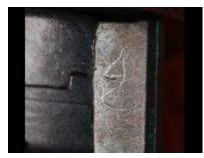
In most forms of bypass that target the actuator, tool marks on the actuator are distinct. In this photo, we see tool marks on the actuator of a Code Lock (4000 series). Notice tool marks are at a variety of angles and depths, all of which are inconsistent with normal use or wear.
