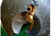
The face of a lock that has seen moderate to heavy use will have many dents and imperfections caused by normal use. How many times have you went to unlock a door and slightly missed the keyway? In the photo, many small dents and scratches from normal use are visible.
