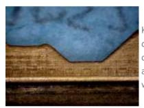
Keys can be duplicated in many ways, but the most common is duplication by hand or with a key machine. Identifying an original vs. duplicate key is an important function of the forensic locksmith. In addition, the forensic locksmith may be able to determine if the key was recently duplicated.
