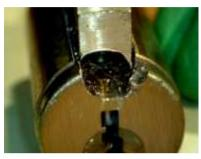
Drilling, a form of shearing, is the most common method of destructive entry against all types of locks. It is frequently used by locksmiths to remove locks when they cannot be opened non-destructively. In this photo, the plug of a KIK cylinder has been drilled at the shear line, allowing the plug to freely rotate.
