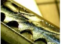
Drills are much like firearms in terms of forensic evidence. Bullets fired from a gun have striae based on the barrel used; the same goes for drill bits used in destructive entry. In the photo, the spiral striae left by the drill bit can clearly be seen in the plug of the lock.
