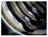
In this photo we see the cylinder from the failed bumping of an EVVA 3KS. The serious damage to the walls of the cylinder is due to the wafers slamming against the cylinder when bumping was attempted.
