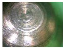
Up close we can see that the ring is actually due to the milling marks starting to be removed and lightly polished. The pin has also been slightly distorted in the very center, also due to the key making contact with it.
