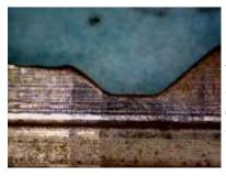
In this photo, the duplicate key is shown. Notice that the ramps and valleys of the key are slightly different than the previous photo. In addition, we see that the key is nickel-silver plated, with no plating on the cuts. Depending on the factory-original specifics, this may also indicate that it is a duplicate key.
