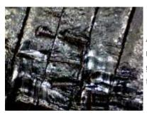
A closer inspection of the tool mark shows a series of parallel teeth marks, probably from the use of a plumber's wrench or tongue-andgroove pliers. Marks can be used in tool mark comparisons done with tools found in a suspect's posessions.
