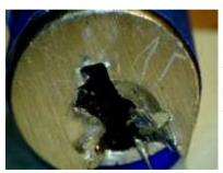
Heavy damage to the face or keyway of the lock can mean many things. A thorough investigation of tool marks, including angles and positions, helps to reveal how entry was accomplished. In this photo the keyway has been considerably widened and gouged so a tool can be inserted, probably a screwdriver or chisel.
