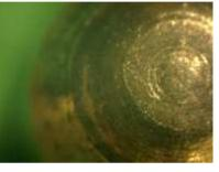
What is most interesting is that pin 5 (the furthest back) has considerably less wear, and more visible scratches. This all makes sense; it is only touched by the tip of the key, and the tip of the key is the most worn down because it makes contact with all of the pins.
