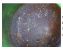
A closer examination can confirm the use of nitric acid by identifying trace evidence left by the chemical reaction between nitric acid and brass. The scattered blue particles are cupric nitrate and zinc nitrate, a byproduct of the chemical reaction.
