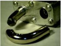
Many destructive attacks against low security padlocks break the shackle because, relative to the body, it is the weakest component. In this photo, the padlock shackle is broken in two places, with one piece being stuck beneath the locking bolt.
