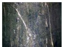
Like the bottoms of the pins, the sides can tell a great deal about the skill level of the attacker. In this photo, gouges on the sides of the keys are rather deep, caused by extreme force being used on both the tension and picking tools. With this much material removed, it may be possible to identify pin material on a suspect's possessions.
