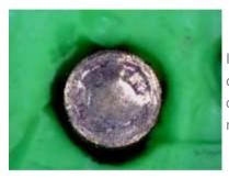
In some pin designs the bottoms of the top pins will be considerably damaged by bumping. In this case, the bottom pins are lightly rounded on both sides, allowing them to be inserted either way. When bumped repeatedly, the bottoms of the top pin become considerably dented.
