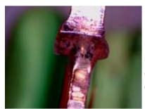
In many covert entry techniques a key is used as a tool to affect entry. Keys with unusual marks or deformations can provide clues as to their use or intended purpose. In this photo, the shoulder of the key is deformed and compressed. This happens to be a bump key's shoulder, caused by impact against the face of the lock.
