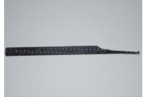
Carbon fiber lockpicks were considered for use in <u>Anti-Forensics</u>, but my research shows that they leave marks similar to traditional metal lockpicking tools. The photo shows a finished carbon fiber lockpick in the half-diamond design. This pick is roughly 0.025" thick.
