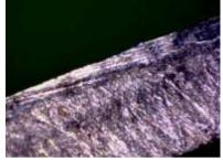
When a key is duplicated with a stylus-based key machine a mark is left on the side of the original key. This is due to the stylus being gently dragged against the key, and resembles a long, straight, polished line. This cannot be confused with wear of the key because it is not in the direct center of the key.
