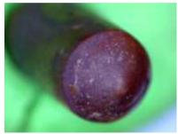
Chemicals are powerful because they can fundamentally alter metals to leave them vulnerable to many other attacks. In this case, brass pins are dark red/brown because of  $NO_2$  fumes released when concentrated nitric acid contacted the brass components. Nitric acid has the effect of eating away the copper in brass.
