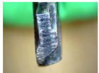
The key has also started to show signs of wear, mostly in the center where the pins have been touching it. In this particular case, wear resembles a staircase pattern. In addition, the key has picked up more lubricant, making the line on the key considerably darker.
