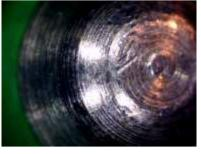
The marks left by a pick gun are so distinct, compared to the rest of the pin, that is is often possible to count them to determine how many times the pick gun was triggered. Each time the needle strikes, the bottom pins may rotate slightly, allowing marks to be separate and distinct.
