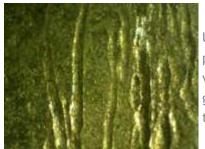
Up close we can see the very distinct markings left on the cam by the pick gun needle. These marks are well defined and would make for a very good tool mark comparison. Because they are so deep, the pick gun needle may also have material residue that can be linked back to this cam.
