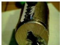
In addition to damage to the keyway, the upper pin chambers have been completely sheared off, leaving the plug and broken cylinder free to rotate in the lock. This attack appears to be torsion applied counter-clockwise to the plug through the use of a screwdriver.
