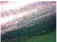
In the case of low-high pinning combinations it is even harder to lift pins without touching the sides of other pins. In this photo, a series of long scratches travel up the side of the pin. Interestingly, we may be able to measure the length of scratches to determine if the attacker raised the adjacent pin high enough.
