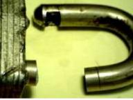
In this photo, the body of the padlock shows tool marks in places where the hammer impacted the lock. The crescent shaped marks are numerous and can be measured to determine the size and shape of the hammer used. At least three different points of impact are visible.
